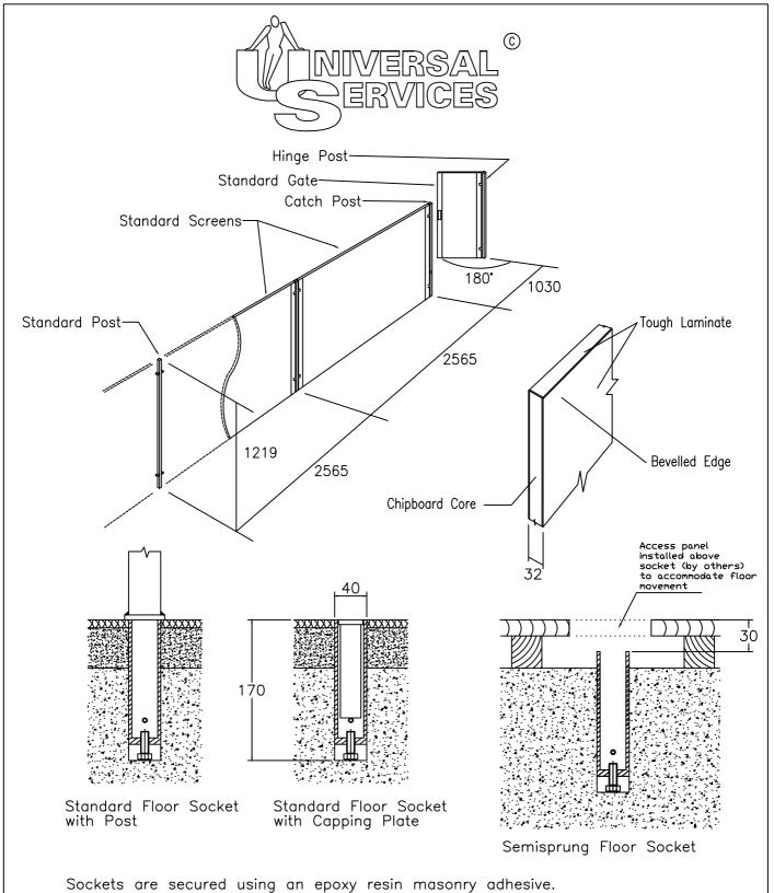
Sockets are secured using an epoxy resin masonry adhesive The screw provides fine adjustment to level the socket until the adhesive has cured.
